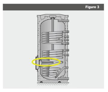
Subsequently, to achieve a longer service interval between anode replacements and to provide additional protection of the tank, a second (lower) anode rod was incorporated into PQN-03 Product Quality Notice
