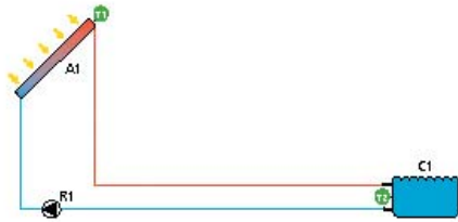
Direct flow-through, intelligent pump control
