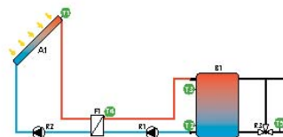
External heat exchanger, intelligent pump control, heating return increase
