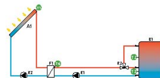
External heat exchanger, zone loading, intelligent valve control
