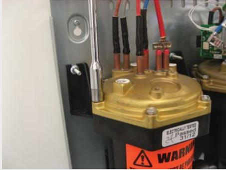
**i** Place a cloth or absorbent paper under the heating module to catch any water that leaks from the vessel when the brass head is removed.
