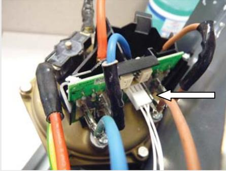
2. Unplug the ¼" push on connectors for the black, brown, and grey (grey is only for 27/36kW units) wires connected to the triac boards on the top of the heating module (Fig. 3). These are the wires that go from the white terminal block on the right side of the unit to the triac boards mounted on the brass top of the module. Wiring can now be placed out of the working area.
