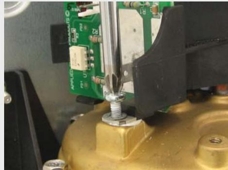
2. Lift up and remove the moulding complete with the printed circuit boards (Fig. 5). Feed the 3 or 5 wires through the holes, noting which color wires go through the large and small holes for reassembly.
